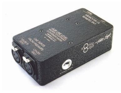
The Sonic Orbit converts "center/sides" (mid-side) line level signals into left/right (X/Y) stereo. This decoding matrix goes between mic preamps and a recording device.
